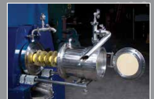
Rail system allows for easy maintenance and tank removal.
