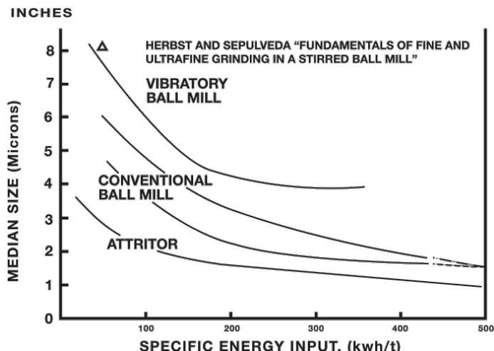
Comparison of the effectiveness of various grinding devices for ultrafine grinding of Pima chalcocite concentrate. Herbst and Sepulveda, "Fundamentals of Fine and Ultrafine Grinding in a Stirred Ball Mill," Proc. Powder & Bulk Solids Conf., Chicago, IL, May 1978.
